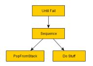
Using an Until Fail repeater, we can repeatedly pop an item from the stack and operate on it, until the point the stack is empty, at which point PopFrom-Stack will return a fail and exit out of the Until Fail repeater.
